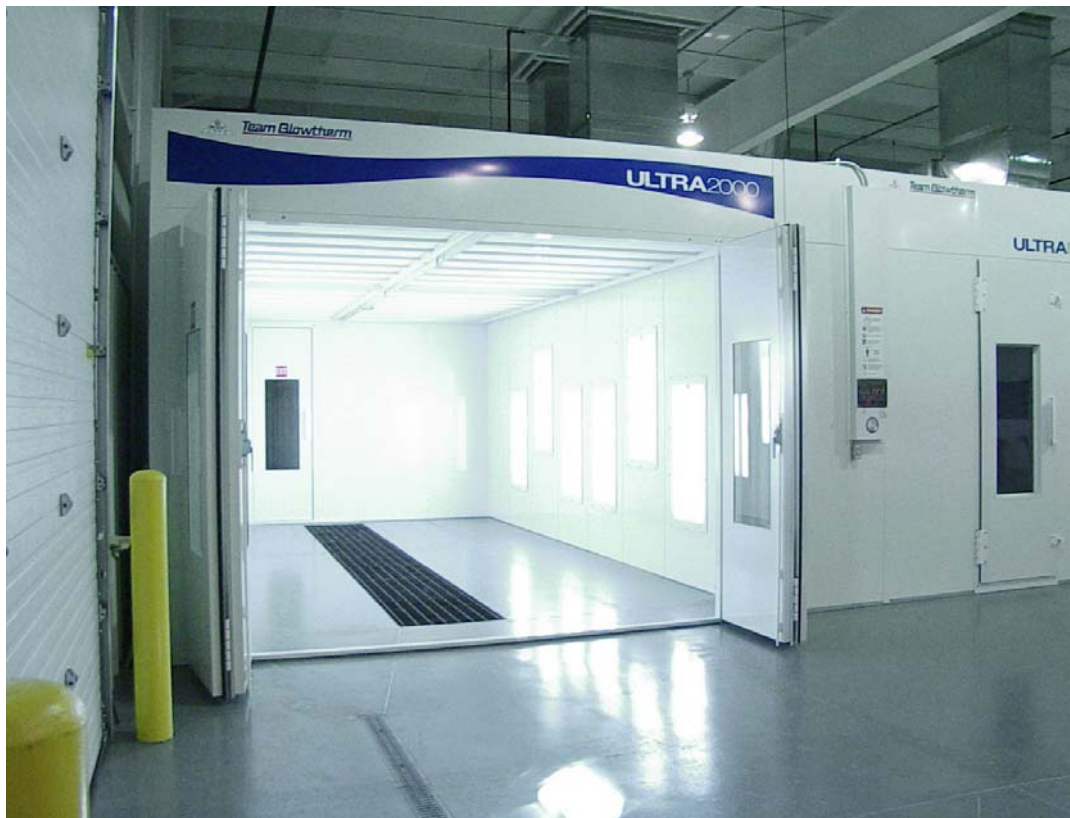
Pit Style Downdraft with attached Paint Mix Room
